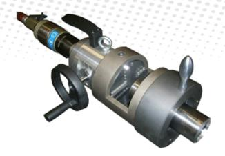
The pneumatic or electric powered **SE-Series** end prep tools are lightweight and portable. They will perform repeatable quality weld preps on most metal pipes and tubes including stainless steel, from 10 mm to 120 mm OD. The cutting head will bevel, face and counterbore individually or in a simultaneous operation. The tool-holder plate can hold up to 4 tool blocks.
